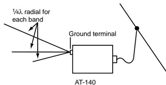
$\frac{1}{4}\lambda$  (quarter wavelength) radial for each band is suitable for a counterpoise. Install the counterpoise directly below the AT-140's ground terminal. Insulate the ends of each radial from other metal objects. Lay-out the radial horizontally and as straight as possible.
