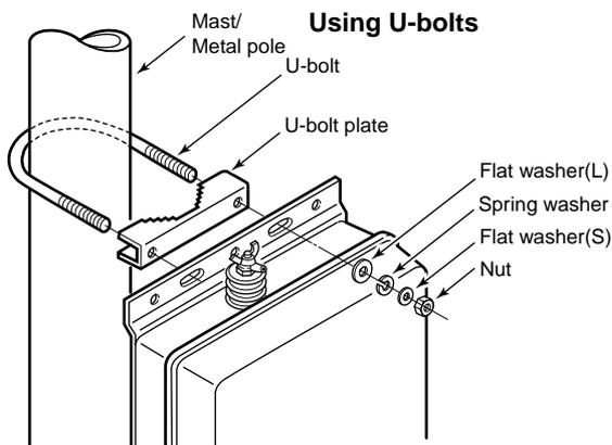
**WARNING:** Mount the AT-140 securely with the supplied nuts and bolts. Otherwise, vibrations and shocks due to waves, etc. could loosen the antenna tuner making it fall, causing personal injury.
